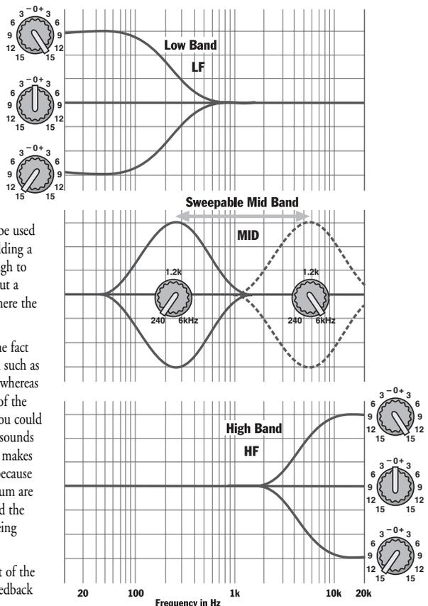
Bearing the above points in mind, the best approach is to use small amounts of boost, especially when working live. EQ cut, on the other hand, causes far fewer problems, and *rather than boost a particular sound it is frequently more rewarding to apply cut in whichever part of the audio spectrum that appears to be overpowering*. In this application, the sweep mid control is also very effective.
