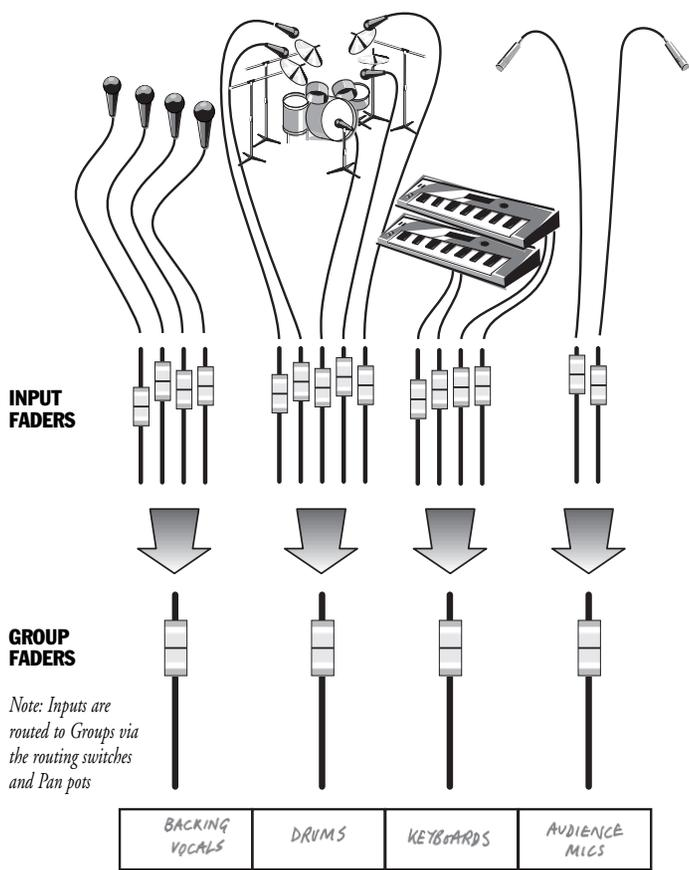
*Note: Inputs are routed to Groups via the routing switches and Pan pots*
